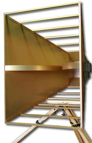
Figure 5 – Double Ridge Guide Horn Antenna
