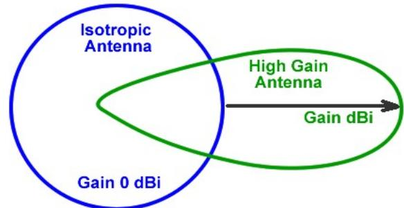
Figure 1 – Antenna Gain dBi
